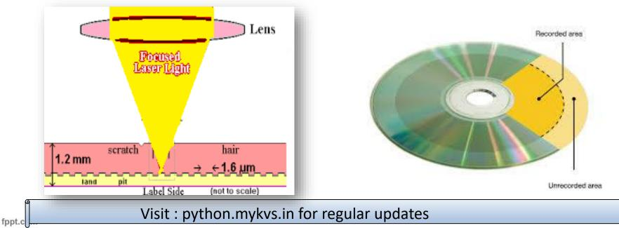
DVD - Short for digital versatile disc or digital video disc, a DVD or DVD-ROM is a disc capable of storing a significant amount more data than a standard compact disc. DVD-ROM drives that utilize these discs were first sold in 1997.Works similar to cd but store data densely due to it's faster speed. DVDs have differing capacities.
